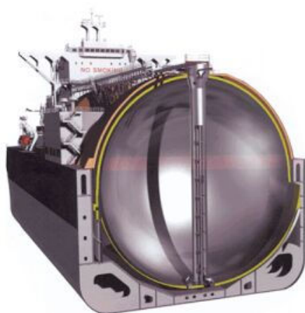
Figure B-29: Principle of cryogenic tankers with Moss tank system (left) and LNG ship as example for cryogenic tank ship (right) (Source: www.statoil.com ).
