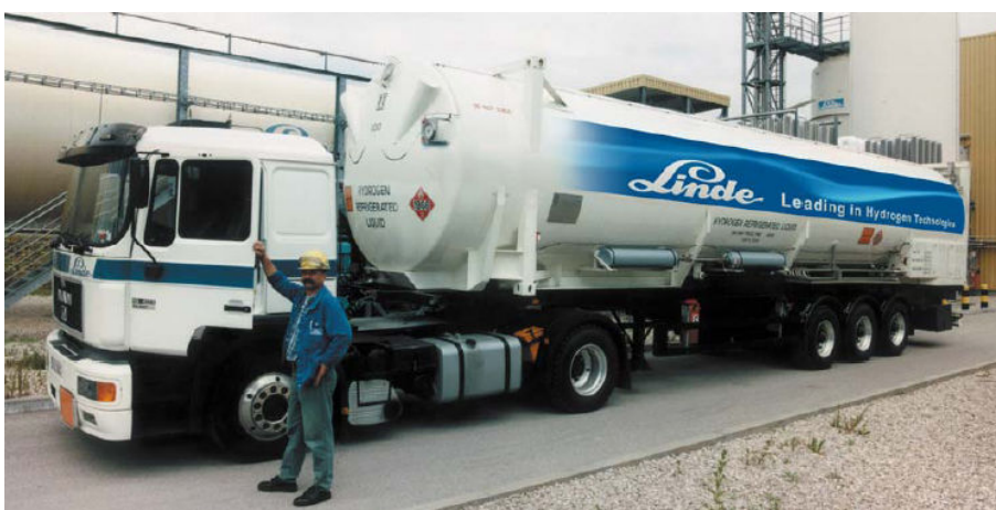
Figure B-28: Articulated train with semi-trailer equipped for liquid hydrogen; (source: Linde AG www.linde-gas.de ).
