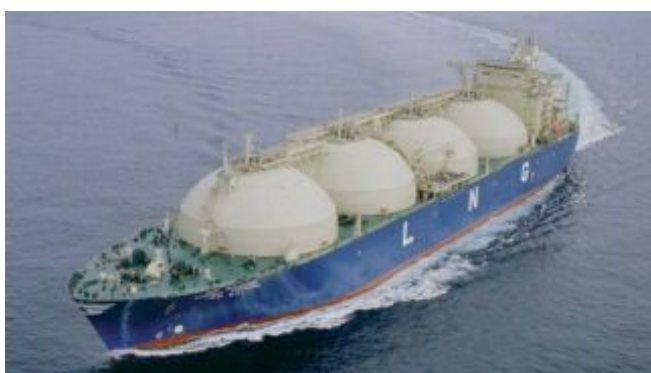
Figure B-29: Principle of cryogenic tankers with Moss tank system (left) and LNG ship as example for cryogenic tank ship (right) (Source: www.statoil.com ).
